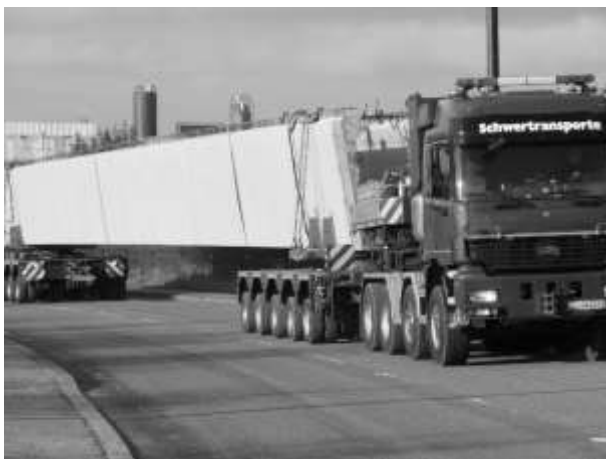
Figure 10. Transport logistics – long span precast beams
