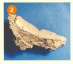
The floor varies in thickness from 30 to 80 mm and was laid on an even base of sandy clay. The concrete has been well compacted and
